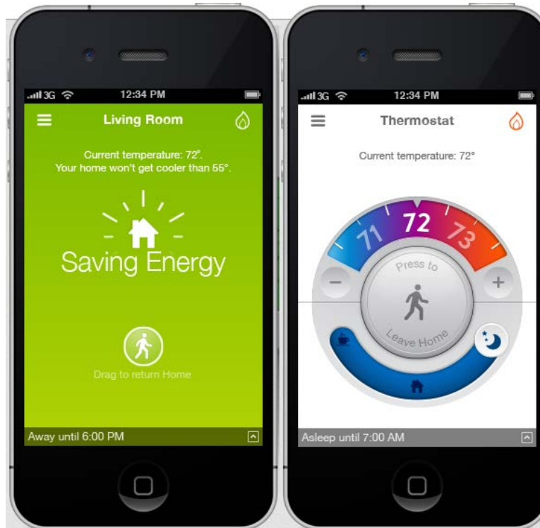
(b) Temporary Overrides: Screenshots of the smartphone app that facilitates changes to the temperature setpoint. The left panel shows the interface after the user indicates she is not home. The right panel shows the same interface when the user indicates she is at home.
