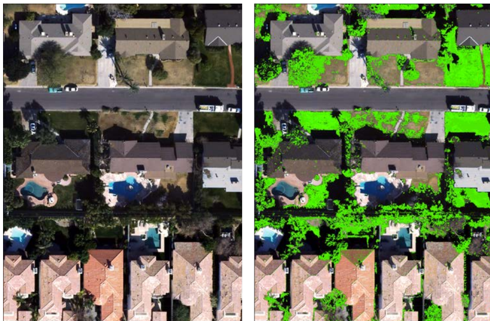
Figure 2: Illustrative remote sensing images demonstrating the classification of green space. Panel A on the right shows what our remote sensing images look like, while Panel B on the left shows how the machine learning algorithm codes the pixels of green space.
